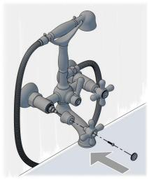
Note: Do not over tighten as this could damage the ceramic cartridge!
