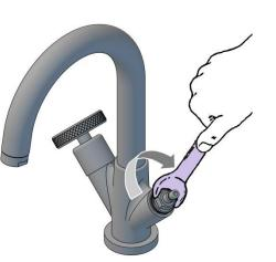
**Note:** Do not over tighten as this could damage the ceramic cartridge!
