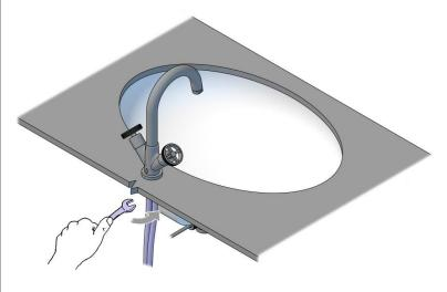
Connect hot and cold flexi tail hoses to water supplies as shown.
