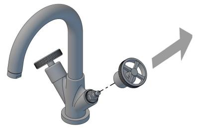
**NOTE**: At any time, should the handle feel loose, retighten the retaining flange.
