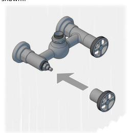
Note: Do not over tighten as this could damage the ceramic cartridge!
