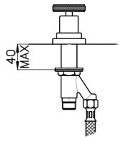
Measure and cut tap holes, with a maximum hole spacing of 110mm from tap body centre line. Overall max hole cut out distance: 220mm
