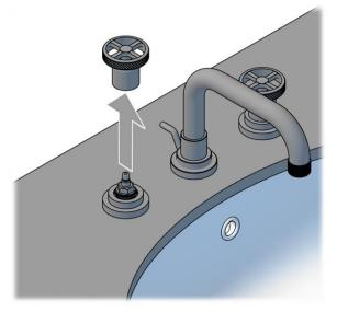
**NOTE**: At any time, should the handle feel loose, retighten the retaining flange.
