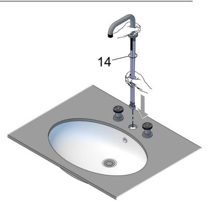
Under the sink, stack the supplied half ring rubber gasket 15, above the half ring mounting plate 16, and feed them onto the stud. Then screw the mounting nut 17, onto the stud. Screw the mounting stud until the half ring rubber mates up with the underside of the sink.
