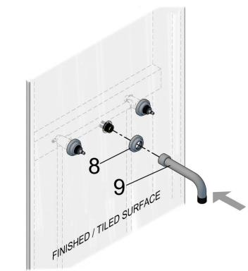
■ Place the cover plate **8**, over the ¾" to ½"adptor. Line-up the thread end of the spout **9**, with the thread of the adaptor. Apply the spout onto the adaptor and screw on until it is firmly secured. Ensure to apply adequate PTFE tape, or a suitable sealing material to the threads to prevent any leakage from the wall spout.
