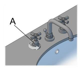
Once totally loose, simply remove the handle from cartridge spline.
