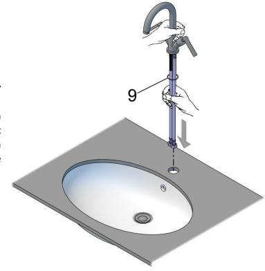
Under the counter top, stack the supplied half ring rubber gasket 10, above the half ring mounting plate 11, and feed them onto the stud. Then screw the mounting nut 12, onto the stud. Screw the mounting stud until the half ring rubber mates up with the underside of the top.
