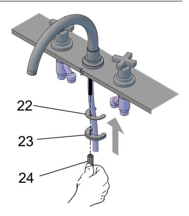
8 • Check the position on the spout body, then tighten the nut using a 13mm spanner or smooth jawed shifter.
