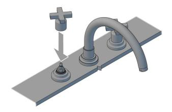
**Note:** Do not over tighten as this could damage the ceramic cartridge!
