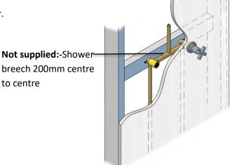
Install the C-tech ¼ turn cartridge 1, into the breech seat 2. Ensure that the base of the cartridge is firmly tightened onto the base of the seat.
