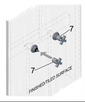
Position the retaining flange 7 with handle, over the cartridge shaft spline, and carefully hand turn the retaining flange onto thread until it is firmly seated.
