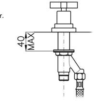
Measure and cut tap holes, with a maximum hole spacing of 110mm from tap body centre line. Overall max hole cut out distance: 220mm
