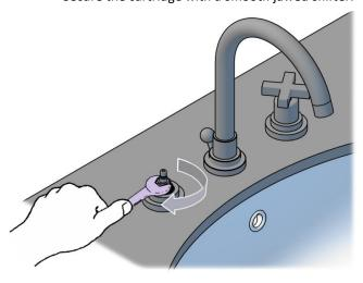
**Note:** Do not over tighten as this could damage the ceramic cartridge!
