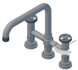
Once totally loose, simply remove the handle from cartridge spline.
