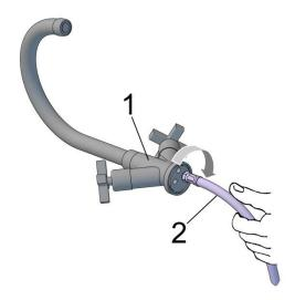
Install the water supply hoses 3, into the tap body - 1
