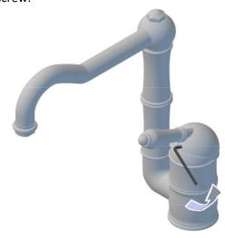
Lift the and carefully remove the dome from the cartridge lever arm.
