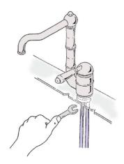
Check the position on the sink of the tap, then tighten the nut using a 13mm wrench.
