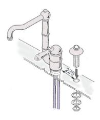
Insert the hand spray escutcheon into the sink hole
