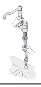
Insert the tap into mounting hole. Feed the water supply hoses carefully through the hole ensuring that they are not bent or kinked, as this could result in permanent damage or leakage.
