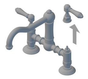
**NOTE**: At any time, should the handle feel loose, retighten the retaining flange.
