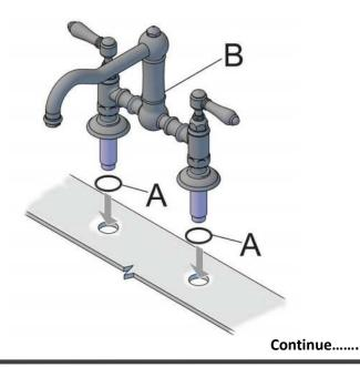
Insert the tap **B**, into work top mounting holes.
