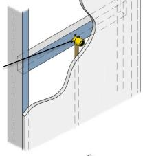
Install the connector pipe 1, into the wall elbow connector. Ensure that the pipe is adequately sealed using PTFE tape or appropriate sealing material to ensure a water tight connection.
